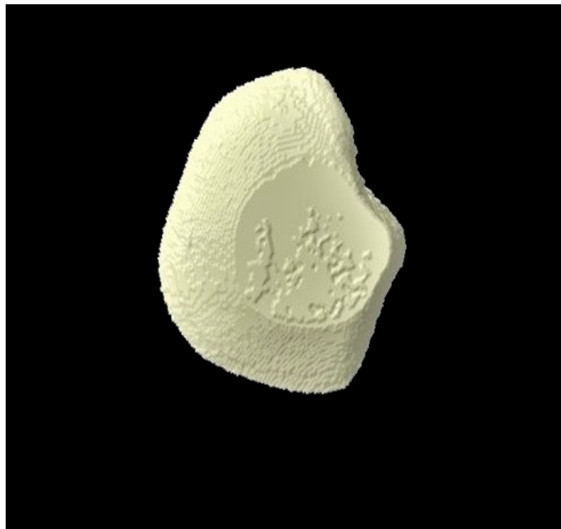
Figure 9. Micro-CT image of group 3 samples presenting enamel surface post-demineralization.
