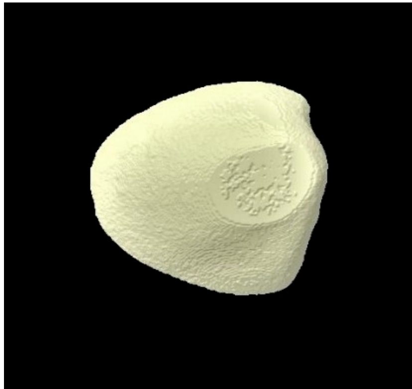
Figure 6. Micro-CT image of group 2 samples presenting enamel surface post-demineralization.
