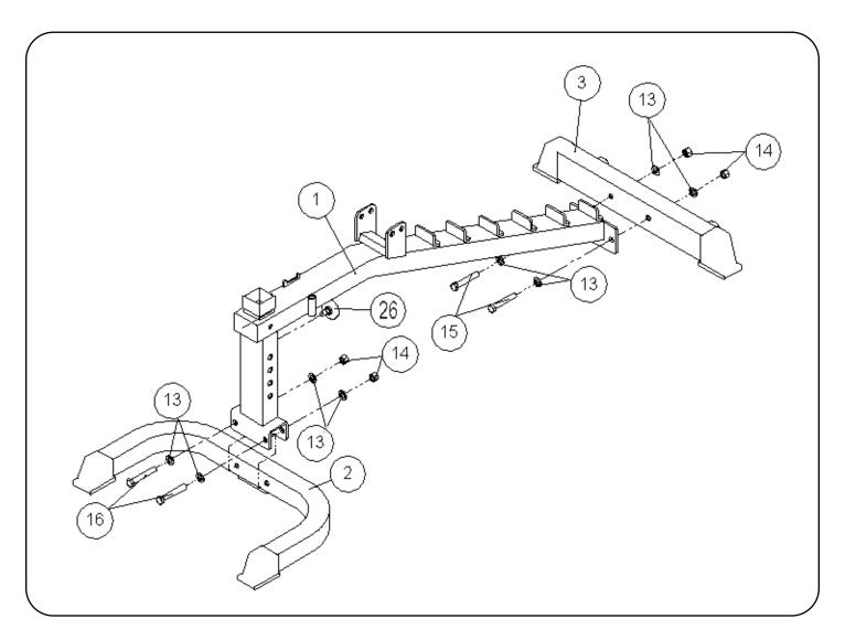
**STEP 1** Connect Main Frame (1) to U Front Base (2) with Bolts (16), Washers (13) and Nylon Lock Nuts (14).
