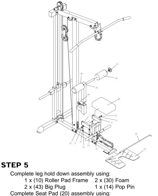
Slide L Pin (22) through holes in Foot Plate (11) and Main Base (1).
