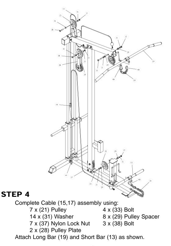
NOTE: Hand tighten bolts and nylon nuts until machine is fully assembled.
