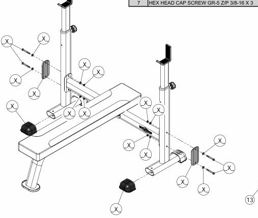
Remove the hardware labeled with X from the **ROB-311** to allow the attachment of the **ROB-311SS Olympic Bench Safety Spotter.**
