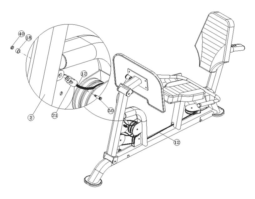
Step 10 Assembly of Leg Press Cable to AXT-2S\_AXT-2D Unit
