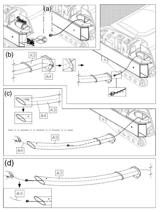
1-3. Hold the data cable at the top of the right pedestal (A3), and insert the bottom of the pedestal onto the pedestal mount. Avoid pinching or crimping the data cable. Place the water guard (A5) on the pedestal higher than the motor cover. Loosely secure the right pedestal (A3) with screws (41). Insert the left pedestal (A7) onto its pedestal mount, and loosely secure it with screws (41). Do not tighten screws. Make sure the pedestals can still move slightly.
