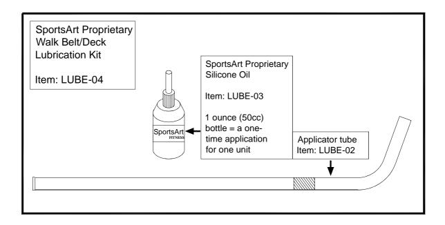
Periodic lubrication of this treadmill walk belt is so important that lubricant is provided with this treadmill. More lubrication kits can be found by contacting SportsArt Fitness.
