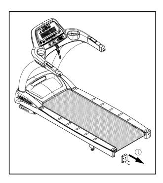
2. Remove screw covers and screws from the left landing strip. Then remove the left landing strip.
