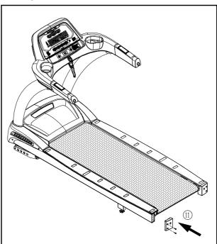
12. Note: The physical task of lubricating the treadmill can be done at any time. To activate the lubrication mode, when the start up banner, SPORTSART-XXX, is displayed, simultaneously press and hold INCLINE + INCLINE + 0 keys for two seconds. The treadmill motor will operate at low speed, allowing you to lubricate the walk belt and deck. To exit lubrication mode, when the message "PLEASE PRESS THE STOP KEY AFTER FINISHING LUBRICATION" appears, press the STOP key.
