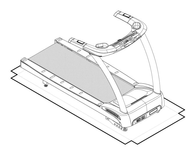
1-1. Remove screws (41) from the pedestal mount area. Inspect whether the screw sockets in areas A and B are in place on the product. If not, remove them from the hardware kit and insert them into place on the product.
