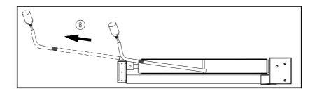
9. Secure the left metal bracket back into place. Note that the metal bracket must be above the walk deck and below the walk belt. And it must press against the rear roller axle as shown..
