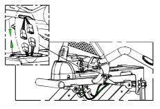
3. Secure the handlebar with washers and screws.
