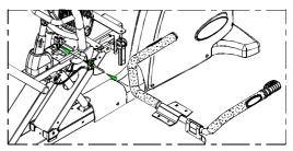
2. HTR handlebar wires are marked left and right. Match them to wires extending from the frame.
