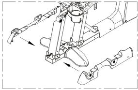
2. Loosely secure each screw. After all screws are in place, tighten them down.
