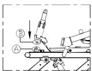
3. Secure the gas spring with the pin and R clip.
