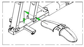
2. Loosely secure each screw. After all screws are in place, tighten them down.
