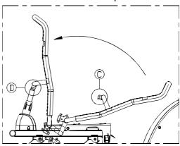
3. Insert the pin and R clip to secure the seat back.
