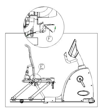
2. The gas spring will push the seat up so that the handlebar and lower covers can be installed. Release the handle after the seat stops moving.
