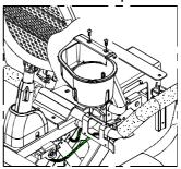
2. Insert a screwdriver through the slots in the cup holder and secure the side screws.
