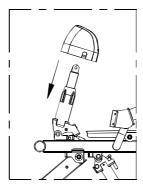
2. Tighten the screws to secure the cover.
