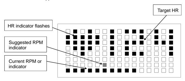
The default startup resistance level is LEVEL 1. Suggested speed is 50 RPM. Actual heart rate is shown on the display. When the workout time is reached, the unit enters COOL DOWN mode.
