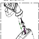
3. After connecting data cables, insert the pedestal into the unit frame. Secure screw/washer set B, then secure set A and set C.
