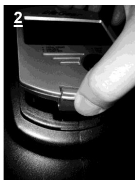
2 Remove the computer from the console.
