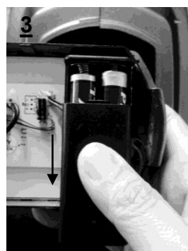
3 Remove the battery cover and place two size AA batteries into the battery housing.
