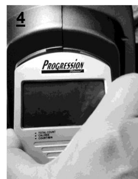
4 Re-install the battery cover and press the computer into position on the console.
