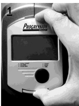
1 Push the tip of the computer.
