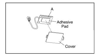
3. Then, reattach the compartment cover to the back of the Control Console (75).
