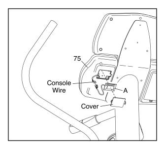
2. Remove the paper from the adhesive pad on the back of the receiver (A). Press the receiver onto the inside wall of the compartment cover.
