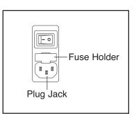
Then, replace the fuse holder and plug the power cord into the jack.
