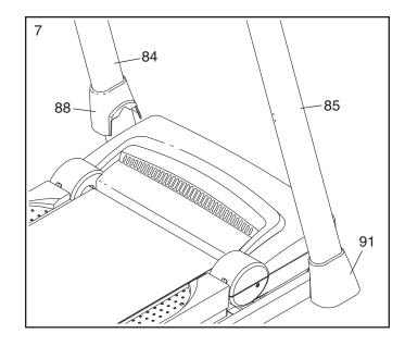
Slide the Right Upright Cover (86) onto the Right Upright (85). Remove the tie from the bracket on the Right Handrail (83). If necessary, press the 5/16" Cage Nuts (38) back into place.
