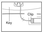
console. After a moment, the displays will light. **IM-PORTANT: In an emergency, the key can be pulled** from the console, causing the walking belt to slow to a stop. Test the clip by carefully taking a few steps backward; if the key is not pulled from the console, adjust the position of the clip.
