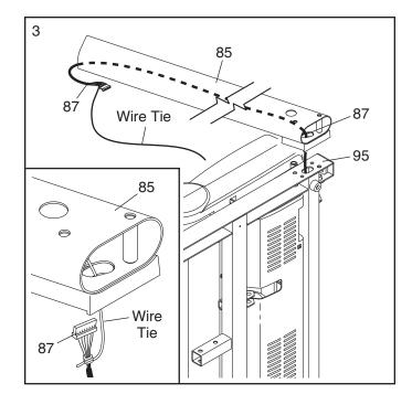
Hold the Right Upright (85) against the Base (95). Be careful not to pinch the Upright Wire (87). Insert two 3/8" x 4" Patch Bolts (7) with two 3/8" Star Washers (11) and a 3/8" x 1 1/2" Bolt (14) with a 3/8" Star Washer (11) into the Right Upright.
