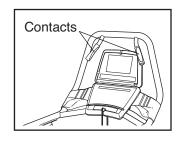
must be resting on the upper contacts, and your fingers must be touching the lower contacts. **Avoid moving your hands.** When your pulse is detected, the PULSE indicator above the display will begin to flash, and then your heart rate will be shown. For the most accurate heart rate reading, hold the contacts for at least 15 seconds without moving your hands.
