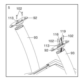
5. With the help of a second person, set the handrail assembly onto the top of the Uprights (93). Make sure that the 5/16" x 1 3/4" Bolts (113) are inserted into the indicated holes in the bottom of the handrail assembly (only one side is shown). Be careful not to pinch any wires.
