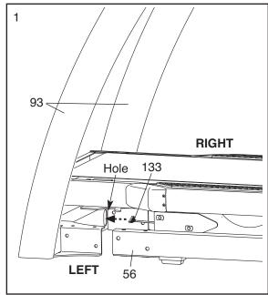
2. Locate the Frame Wire Harness (133) and Upright Wire Harness (119) in the Upright (93) access hole.
