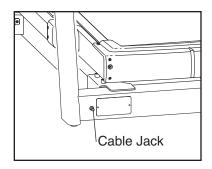
A satellite receiver, VCR, or DVD player can also be connected to the incline trainer. Connect a CATV cable from the coaxial output on your equipment (usually labeled TV OUT or RF OUT) to the cable jack on the front of the incline trainer.
