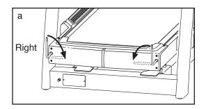
b. If the walking belt has shifted to the left: Remove the key and unplug the power cord. Using a 7/32" hex key, turn the roller adjustment bolts in the directions shown, 1/4 of a turn each. Be careful not to overtighten the walking belt. Then, plug in the power cord, insert the key, and use the incline trainer for a few minutes. Repeat until the walking belt is centered.
