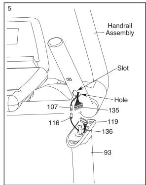
6. Connect the Upright Wire Harness (119) and Console Wire Harness (135). See the inset drawing. The connectors should slide together easily and snap into place. If they do not, turn one connector and try again. IF YOU DO NOT CONNECT THE CONNECTORS PROPERLY, THE CONSOLE MAY BECOME DAMAGED WHEN YOU TURN ON THE POWER. Connect the Upright TV Cable (116) and Console TV Cable (107). Insert the wires downward into the right Upright (93).
