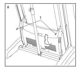
Lower the treadmill (see HOW TO LOWER THE TREADMILL FOR USE on page 29). Remove the three #8 x 3/4" Screws (1). Carefully pivot the Motor Hood (71) off.
