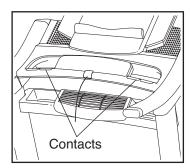
To measure your heart rate, stand on the foot rails and hold the pulse bar with your palms on the metal contacts for approximately ten seconds; avoid moving your hands. When your pulse is detected, your heart rate will be shown. For the most accurate heart rate reading, continue to hold the contacts for about 15 seconds.
