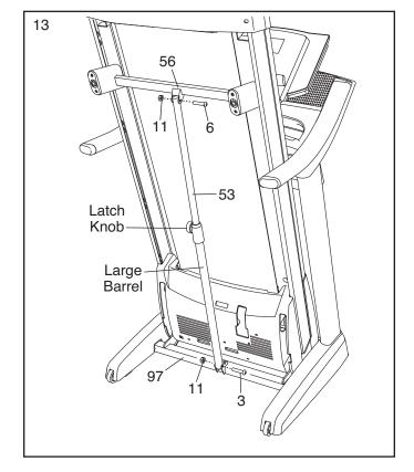
14. Lower the Frame (56) (see HOW TO LOWER THE TREADMILL FOR USE on page 29).
