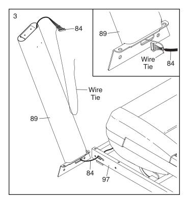
4. Hold the Left Upright (89) against the Base (97). Be careful not to pinch the wires. If necessary, position the Base Ground Wire (94) in the hole in the side of the Left Upright. Insert two 3/8" x 2 3/4" Bolts (7) and two 3/8" x 1 1/4" Bolts (8) with two 3/8" Star Washers (12) into the Left Upright.
