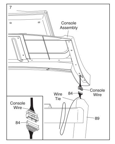
Connect the wire from the Fan Tray (30) to the wire from the console assembly. The connectors should slide together easily and snap into place. If they do not, turn one connector and try again. IF YOU DO NOT CONNECT THE CONNECTORS PROPERLY, THE CONSOLE MAY BECOME DAMAGED WHEN YOU TURN ON THE POWER.
