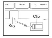
into the console. IMPORTANT: In an emergency, the key can be pulled from the console, causing the walking belt to slow to a stop. Test the clip by carefully taking a few steps backward; if the key is not pulled from the console, adjust the position of the clip.
