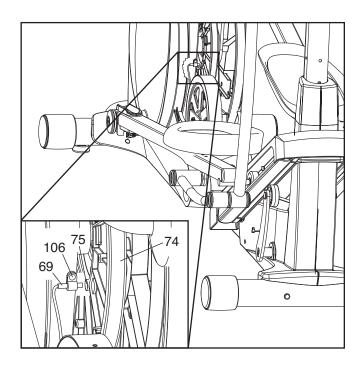
Next, loosen, but do not remove, the indicated M4 x 16mm Screw (106). Slide the Reed Switch (69) slightly toward or away from the Pulley Magnet (75). Then, retighten the Screw.
