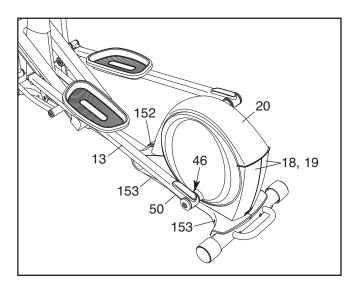
Next, lift the Latch (50) on the underside of the Left Pedal Arm (13), and then lift the Left Pedal Arm off the left Pedal Arm Sleeve (46).
