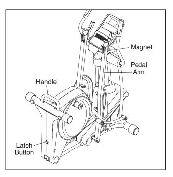
To use the elliptical, first hold the handle, press the latch button, and lower the frame.
