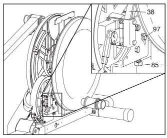
When you are finished, reattach the left shield, replace the left pedal arm, and reattach the access cover. Then, plug in the power cord.
