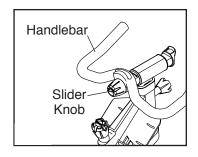
HOW TO ADJUST THE HANDLEBAR POST
