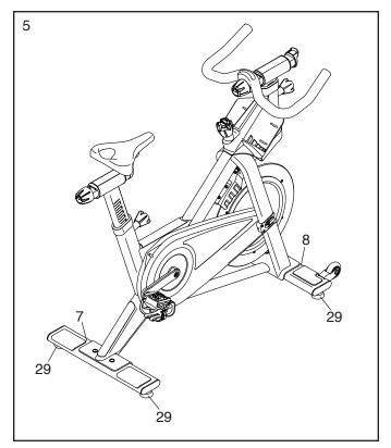
6. Make sure that all parts are properly tightened before you use the exercise bike. Note: After assembly is completed, some extra parts may be left over.
