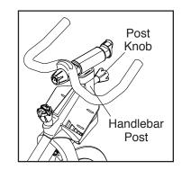
Make sure that the post knob is engaged in an adjustment hole. IMPORTANT: Do not adjust the handlebar post beyond the stop mark on the handlebar post.
