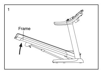
2. Raise the frame until the storage latch locks in the storage position. CAUTION: Make sure that the latch handle locks.
