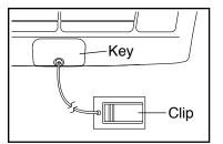
into the console. After several seconds, the displays will light. **IMPORTANT:** In an emergency, the key can be pulled from the console, causing the walking belt to slow to a stop. Test the clip by carefully taking a few steps backward; if the key is not pulled from the console, adjust the position of the clip.
