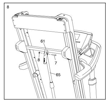
8. Raise the Frame (61) to the position shown. Have a second person hold the Frame until this step is completed.
