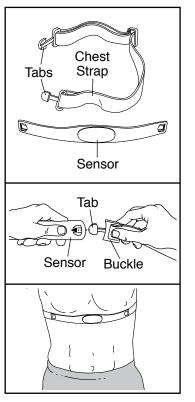
side-up. Then, attach the other end of the chest strap to the sensor. Adjust the length of the chest strap, if necessary.
