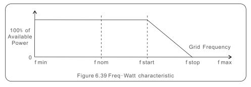
Over frequency load shedding Fstart range 60~62Hz, default setting 60.2Hz
