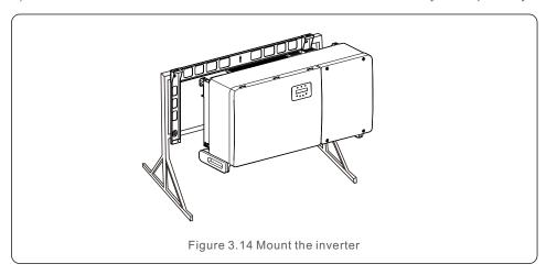
5) Use supplied 2 M6x12 hex bolts to secure the inverter to the bracket (see figure 3.8).
