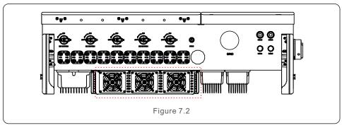
6. Disconnect the fan connector carefully and take out the fan.
