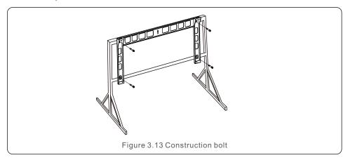
4) Lift the inverter above the bracket and then slide down to make sure they match perfectly.
