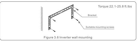
4. Lift the inverter and hang it on the bracket, and then slide down to make sure they match perfectly.
