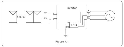
The Anti-PID module repairs the PID effect of the PV model at night. When operating, the inverter LCD screen displays "PID-repairing" information, and the red light is on. The Anti-PID function is always ON when AC is applied.
