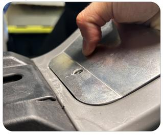
2. Remove the console and using the self tap screw, screw in the bracket, not completly tight but enough to keep it in place and be able to adjust the height.
