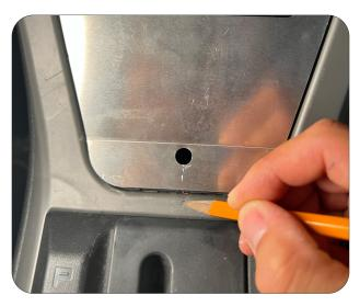
3. Position the mount back on the dash and adjust the bracket until it lets the console sit flush on the dash. Once it sits flush remove the console and tighten the lower bracket.
