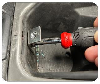
4. Place the mount back in place with switchpro mounted and 12v socket. Alight the lower slot and tighten the M6 buttn head bolt provided to the lower bracket installed on the previous step
