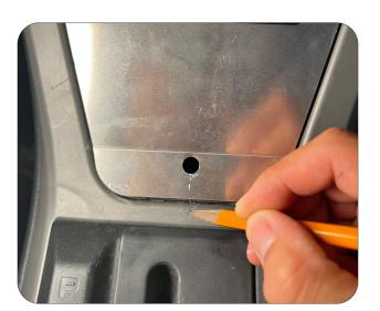
7. Position cosole back on the dash and adjust the bracket until it lets the console sit flush on the dash. Once it sits flush remove the console and tighten the lower bracket.
