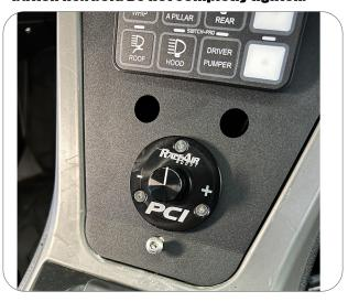
18. Using a small pick punch a small pilot hole to secure the self tapping black head screws provided at the top of the console.
