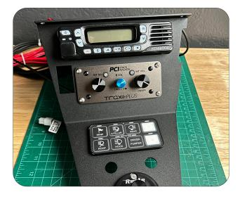
11. The following steps are for Rugged Radios. Install 3 out of the 4 brackets with the hex button head bolts provided. 2 Radios Brackets and 1 Intercom bracket. Do not completly tighten them.
