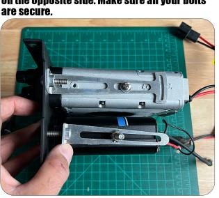
14. Insert the bolts just installed on the intercom into 1 bracket on the console. Add the crush washer and nut . Do not tighten,
