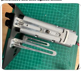
13.Grab the intercom and slide in the hex head bolt through the rear slots of the intercom. 1 bolt on each side.
