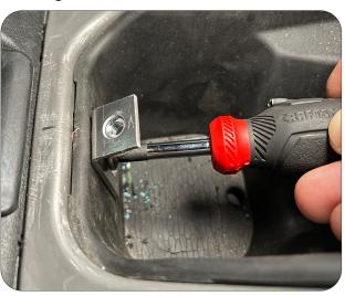
8. If you dont have PCI skip to step 11.Slide PCI intercom through the front of the console. Position the radio cradle on the rear of the console and secure with the 4 hex head bolts and washers. There are 2 on each side
