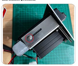
6. Remove the console and using the self tap screw, screw in the bracket, not completly tight but enough to keep it in place and be able to adjust the height.
