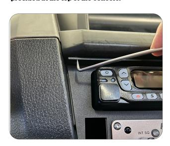
19. Finally tighten the 2 top bolts and the lower console bolt to finish.
