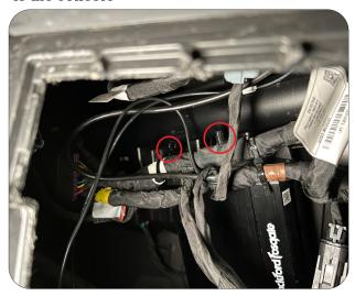
5. Sit the console in place to your liking/position Using a pencil, place a small mark to guide you on where to position the lower mounting bracket
