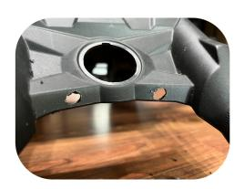
2. Unbolt the lower factory bolts and mount the console sliding in the 2 tabs to the 2 holes drilled in the previos step. Bolt back the factory dash bolts and off you go!
