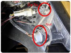
4. Remove the lower Torx screws of the
