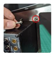
8. With radio secured to your liking, Tighten the 4 locknuts that hold the intercome and radio cradle. 2 on each side, make sure to tighten them ina cris-cross form.
