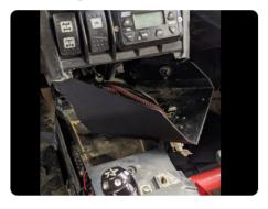
6. Mount the radio cradle to the 4 bolts of the intercom and secure with the lock nuts provided. Leave some play to be able to slide the cradle left and right to fit the radio
