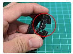
10. Once you mount your switchpro with the brackets that come with the switchpro, mount the start button and make sure the knotch you made lines up with the switchpro bracket
