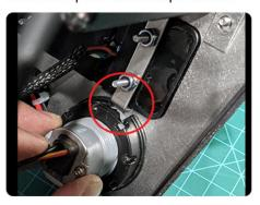
13. Using the T-30 screws from the original plastics, secure the complete mount with radios to the canam.
