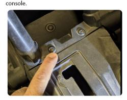
7. Grab your Kenwood/Icom and slide in the radio from the rear of the console and secure with the bolts/lock washer provided, Slide the radio to the distance you prefer, and tighted.
