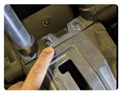
7. Grab the new mount and the radio bracket supplied and mount the intercom to the console using the 4 bolts provided.
