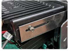
10. With radio secured to your liking, Tighten the 4 locknuts that hold the intercome and radio cradle. 2 on each side, make sure to tighten them ina cris-cross form.
