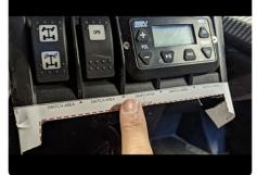
5. Now lets focus on cutting the extra piece for the XL. Us the image as a guide, It would be a square cut around the switch area. You can follow the console lines for an even cut and cut all the way down from your last cut
