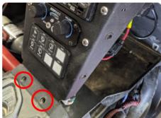
12. Remove the rear panel in the console and using a hole saw, cut the bracket in to be able to route your radio cables. You may needto make a bigger hole depending on wires
