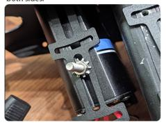
13. Remove the rear panel in the console and using a hole saw, cut the bracket in to be able to route your radio cables. You may needto make a bigger hole depending on wires
