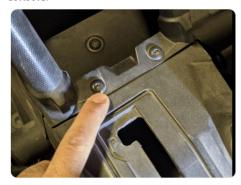
7. Grab the new Mount and the brackets supplied Secure the radio brackets and the intercom to the Mount using the Hex M6 bolts provided. Do not fully tighten just yet.
