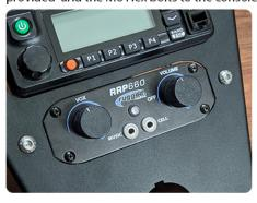
14. Using the T-30 screws from the original plastics, secure the complete mount with radios to the canam.
