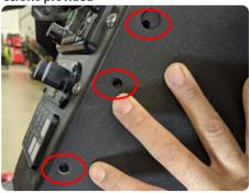
16. Repeat the process for the passenger side dont, remove the factory clip (we all know there a pain) once you have the console and panel bolted together, drill into the factory plastic with the screws provided to secure the rear panel
