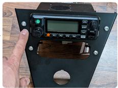
10. On to the intercom, grab the hex head bolts provided and the tooth washer position them in the brackets, and slide in the intercom on both sides.
