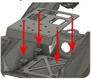
2. Secure the base plate with the 4 self tapping screws supplied
