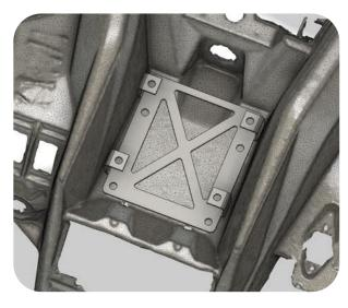
3.Once you have added your device mount go ahead and position the top plate to the mounting slots
