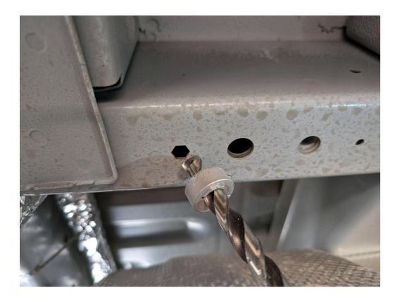
**STEP 3**: Use an 11mm or 7/16" metal drill-bit to enlarge the hole to the correct size for the riv-nut (the Hex works well for the rear strapping).
