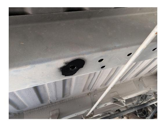
**STEP 4**: Spray paint drill holes to seal the exposed metal.
