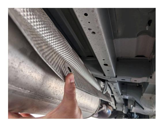
**STEP 1**: Temporarily bend back the heat shield.
