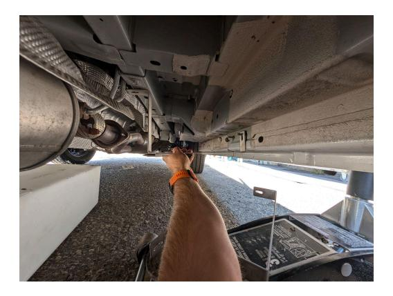
**STEP 2**: Find placement of strapping for top riv-nuts using the center most 8mm factory studs.
