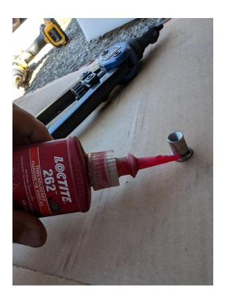
**Tip**: Before installing the riv-nut I add Loctite to the contact point to avoid the t-nut spinning after installation.
