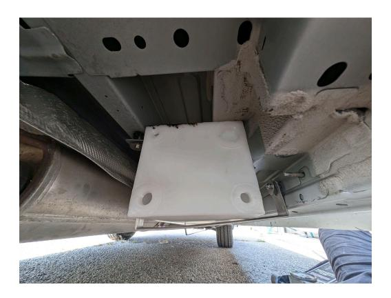
**STEP 6**: Install water tank and bend back the heat shield.
