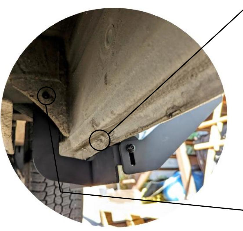
JUSE THE SELF TAPPING SCREWS PROVIDED TO ATTACH BOTTOM MOUNT TO VAN PINCH WELD.
