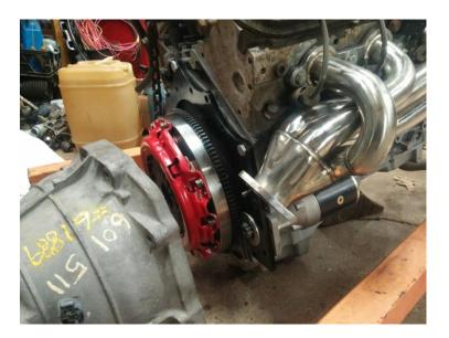
10. Finally, install your Z33 transmission to the adapter plate, now on the back of your LS motor.
