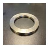
This spacer goes behind the Throwout, or Clutch Release, bearing to shim it closer to the flywheel. Remove cast iron clutch release assembly and remove old bearing. This would be a great time to replace your throwout bearing (SKF Part # N4000). This spacer has a slight press-fit. Using a press and or a vice and large socket, press the spacer onto the cast throwout assembly. Then press on clutch release bearing as shown on page 2.
