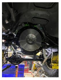
9. Finally, install your Nissan Frontier/Xterra 6 speed manual transmission to the adapter plate using the M12 and M10 bolts
