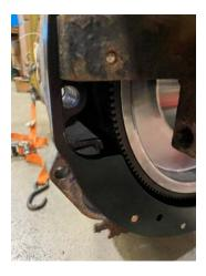
2. In order to fit the starter, the transmission casting boss must be clearanced. Bolt the adapter plate to the transmission and use a permanent or paint marker to trace out where the adapter plate starter hole lands.
