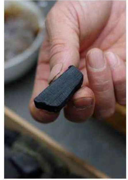
The fine portions are scraped off with a special soft charcoal for lacquering.
