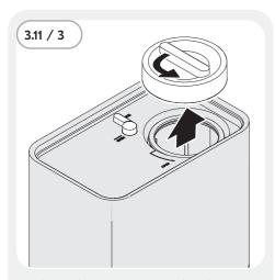
• Open the screw cap off the filter chamber.
