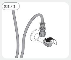
Open the angle valve of the cold water pipe.
