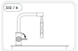
After inserting a new filter, small carbon particles may rub off into the water. The particles do not have an adverse effect on personal health.
