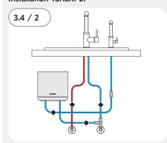
Connection to an auxiliary tap and use of a 2-way tap.
