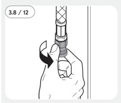
Screw the connection piece (H) or (G) onto the tap for disinfected water by hand.
