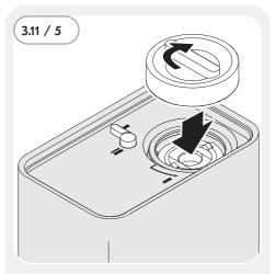
• Turn the screw cap on the filter chamber until it is fully closed.
