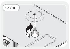
Screw the knurled screw (N) through the wall bracket (C) into the device from below.
