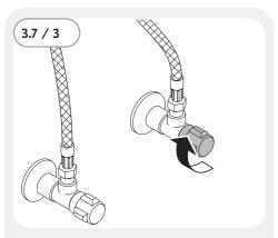
Turn the angle valve on the cold water pipe to close it.
