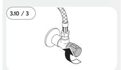
Turn the angle valve on the cold water pipe to close it.
