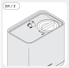
Turn the shut-off valve into the "CLOSE" position.
