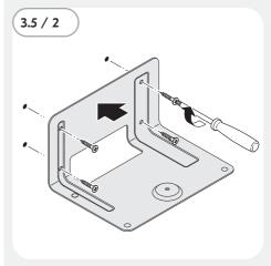
Screw on the wall bracket (C) with the four screws (O).
