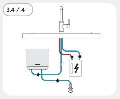
Connection to a 2-way tap and use of a boiler.
