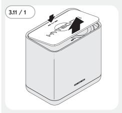
Take off the device cover. To do so, press down on the pressure point and then reach beneath the edge of the device cover.
