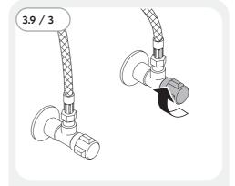
Turn the angle valve on the cold water pipe to close it.
