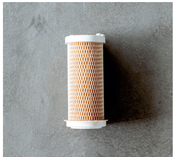
Filter status after 4 months
