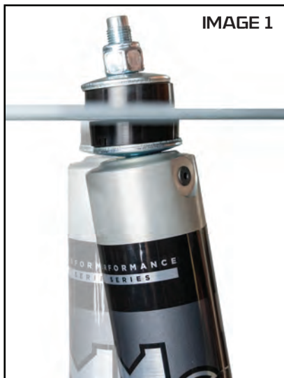
SHOCK SWING NEEDED WHEN SUSPENSION CYCLES
