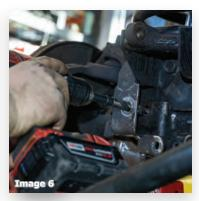
**15)** Now you are at a point you can install all 3 mounting bolts through the main bracket, and into their frame mounting locations.
