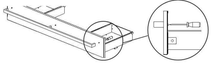
3. To fix handle to the drawer, firstly clear the existing holes from the front using the screws supplied. Insert screw & washer from the inside (back of the draw front) of the drawer, place handle on the outside of the drawer front and secure in two locations. Be careful not to scratch the drawer fronts whilst installing the handles.
