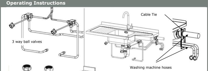
Confirm if the washing machine waste inlet needs to be moved from right to left before securing the unit to the wall. If they do need to be changed see page 6 of these installation instructions.
