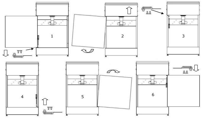
Troubleshooting – Ensure hinge pin is inserted into pilot hole on the door.
