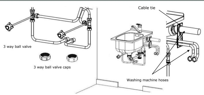
Confirm if the washing machine waste inlet needs to be moved from right to left before securing the unit to the wall. If they do need to be changed see page 6 of these installation instructions.
