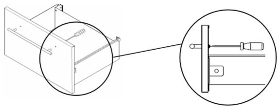
**3.** To fix handle to the drawer, firstly clear the existing holes from the front using the screws supplied. Insert screw & washer from the inside (back of the draw front) of the drawer, place handle on the outside of the drawer front and secure in two locations. Be careful not to scratch the drawer fronts whilst installing the handles.
