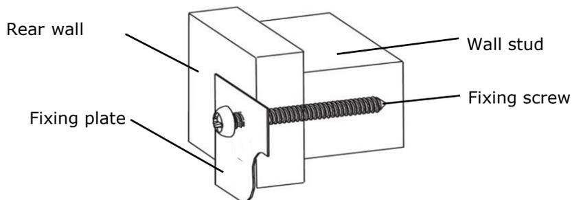
1. Pre drill pilot holes in the positions given (pg 4 - Installation position). Fix the fixing plate using the screws supplied or appropriate wall fixings, check with a spirit level to ensure bracket is level. Tighten screws.
