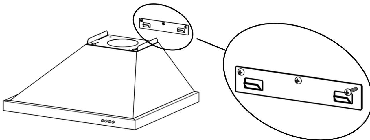
2. Mark the position of the decorative chimney at the ceiling and wall. Cut the cornice moulding away if required, to enable the chimney to sit flush against the wall and ceiling.
