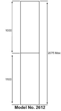
**Note**: When the maximum chimney height is to be used on the extensions, there will be a minimum of 25mm overlap required for top and bottom chimney assembly.
