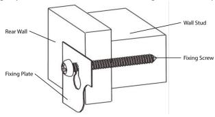
1. Pre drill pilot holes in the positions given. Fix the fixing plate using the screws supplied or appropriate wall fixings, check with a spirit level to ensure bracket is level. Tighten screws.
