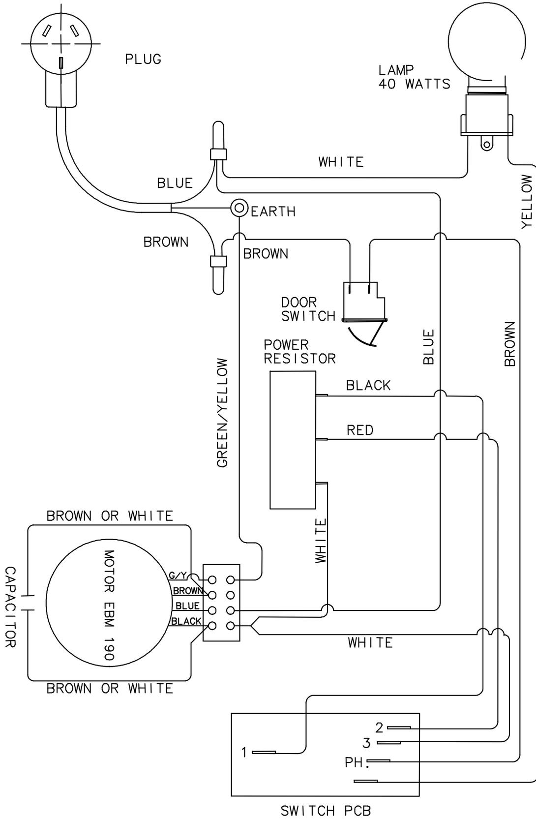
**Wiring diagram - For models manufactured after the 21<sup>st</sup> April 2008**
