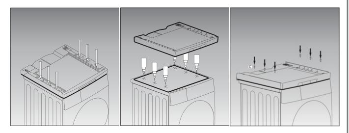
**Step 5:** Install the top panel fixing block (G). Place the top panel fixing block onto the top panel of the washing machine. Align the mounting hole of the block with the mounting hole of the stacking kit, and fix into place using the supplied M6 screw (B) and gasket (D). Do not over tighten.
