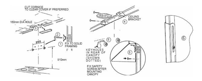
Fix the mounting washers in position, check with a spirit level across the washers to ensure they are level.
