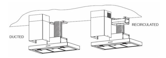
Before drilling any holes check the wall and ceiling are clear of any electrical cables, pipes etc. Fixing to a solid stud is recommended.
