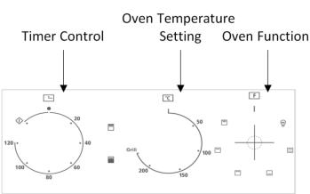
The mechanical timer can be set from 1-120 minutes. To use the timer, the timer knob must be wound up by turning the knob one full turn clockwise then turn it back to the desired time so that the number of minutes on the knob matches the reference mark on the panel. When the timer reaches its off position when coking is complete a buzzer will sound.
