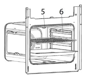
Each appliance comes with a single tray and 2 wire racks. Model RHBO64BX has rack supports moulded into the sides of the oven cavity, whereas RHBO67BX & RHBO69BX have removable wire rack supports. The wire racks have built-in steps, which is a safety feature to warn the user when the rack has been almost fully pulled free of the rack supports.
