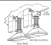
WARNING: The distance between the hob and the mounting holes of the canopy must be at least 880mm for 600&900 model and 900mm for 1201 model to ensure that the fully installed canopy has the recommended clearance of 700mm between the lower part of the hood and the cooking hob. Before drilling any holes check the wall and ceiling are clear of any electrical cables, pipes etc. Fixing to a solid stud is recommended.
