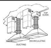
WARNING: The distance between the hob and the mounting holes of the canopy to be at least 855mm for 600 and 875mm for 900 models to ensure that the fully installed canopy has a clearance of 700mm (recommended height) between the lower part of the hood and the cooking hob. 1 Before drilling any holes check the wall and the ceiling are clear of any electrical cables, pipes etc. Fixing to a solid stud is recommended. (1)
