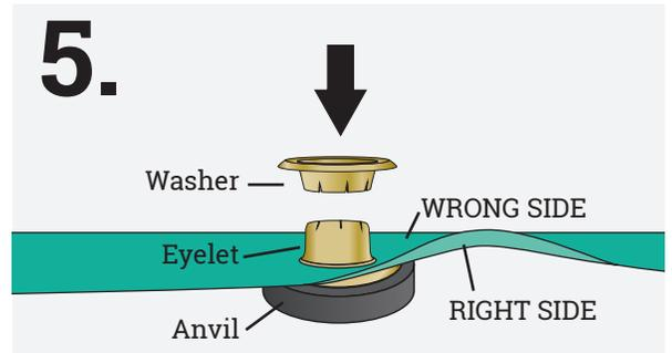
6. Place setter tool into post of front eyelet and hit firmly. Washer and front eyelet will curl together to finish eyelet.
