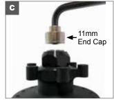
C. Keep 5mm hex wrench in drive side. Thread on the 11mm end cap with another 5mm hex wrench.
