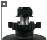
B. Tighten the adjusting nut with dust seal until snug against the bearing. The O-ring inside the adjusting nut provides drag to hold the bearing adjustment.
