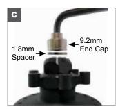
C. Keep 5mm hex wrench in drive side. Place the 1.8mm spacer on the axle and thread on the 9.2mm end cap using another 5mm hex wrench.
