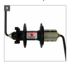
1.Insert a 5mm hex wrench into each end of the silver endcaps (where quick release goes though, one on each side).
