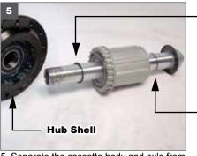
5. Separate the cassette body and axle from the hub shell by grabbing the body with your hand and pulling it out from the drive side.
