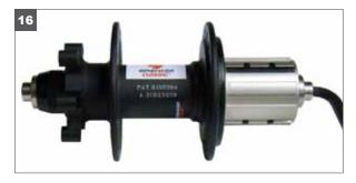
16. Insert the 5mm hex wrench into the cassette side end cap. Holding the hex wrench in place, the knurled adjuster can be used to adjust the play. The internal O-ring will hold it in place, no lock nut is required. This can be done with fingers or with pliers.
