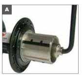
A. Insert 5mm hex wrench into drive side end cap. Keep the 5mm hex wrench in place.
