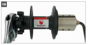
16. Insert the 5mm hex wrench into the cassette side end cap. Holding the hex wrench in place, the hex adjusting nut can be used to adjust the play. The internal O-ring will hold it in place, no lock nut is required. This can be done with fingers or an adjustable wrench.
