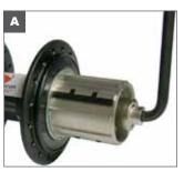
A. Insert 5mm hex wrench into drive side end cap. Keep the 5mm hex wrench in place.
