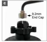
C. Keep 5mm hex wrench in drive side. Thread on the 9.2mm end cap with another 5mm hex wrench.
