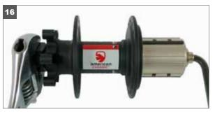
16. Insert the 5mm hex wrench into the cassette side end cap. Holding the hex wrench in place, the hex adjusting nut can be used to adjust the play. The internal O-ring will hold it in place, no lock nut is required. This can be done with fingers or with an adjustable wrench.
