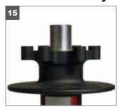
15. When the bare threaded axle is showing, grease threads and then re-install the knurled adjusting nut and end cap.
