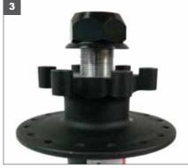
3. Keep the 5mm hex wrench in drive side (side with cassette) end cap to hold the axle in place and unthread the hex or knurled nut with dust seal.
