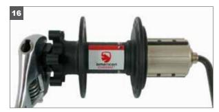
16. Insert the 10mm hex wrench into the cassette side end cap. Holding the hex wrench in place, the hex adjusting nut can be used to adjust the play. The internal O-ring will hold it in place, no lock nut is required. This can be done with fingers or with an adjustable wrench.
