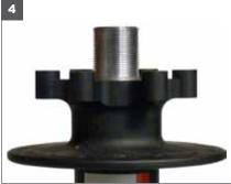
4. Once the end cap and adjusting nut are removed, you are ready to open the hub.
