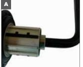
A. Insert 10mm hex wrench into drive side end cap. Keep the 10mm hex wrench in place.
