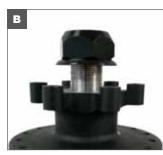
B. Tighten the adjusting nut with dust seal until snug against the bearing. The O-ring inside the adjusting nut provides drag to hold the bearing adjustment.
