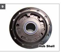
9. Clean out the hub shell for inspection and new grease.
