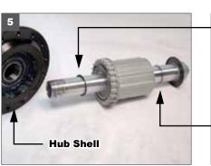
5. Separate the cassette body and axle from the hub shell by grabbing the body with your hand and pulling it out from the drive side. Very Important! Locate the 0.5mm axle spacer, which is either stuck to the drive side hub shell bearing or the inner bearing on the cassette body. This spacer is critical to maintaining the correct engagement, do not lose.
