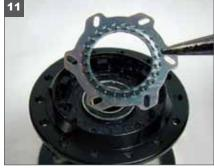
11. With a thin layer of clean grease coating the hub shell, re-install the cam plate. Refer to the picture for the correct orientation. Do not put the cam plate in upside down.
