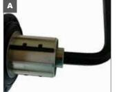
A. Insert 10mm hex wrench into drive side end cap. Keep the 10mm hex wrench in place.
