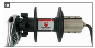
16. Insert the 10mm hex wrench into the cassette side end cap. Holding the hex wrench in place, the hex adjusting nut can be used to adjust the play. The internal O-ring will hold it in place, no lock nut is required. This can be done with fingers or with an adjustable wrench.
