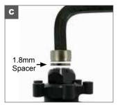
C. Keep 10mm hex wrench in drive side. Place the 1.8mm spacer on the axle and thread on the end cap using another 10mm hex wrench.
