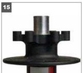
15. When the bare threaded axle is showing, grease threads and then re-install the knurled adjusting nut and end cap.
