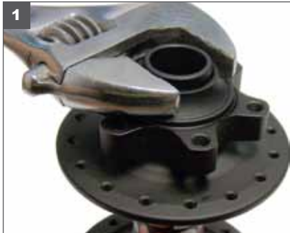
1. Using a 22mm wrench, turn counter clockwise to loosen and remove the large black threaded cap.
