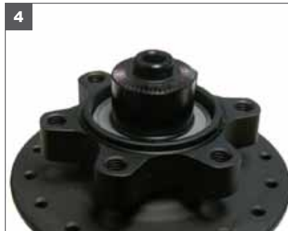
4. Place the Terrain 9mm Quick Release cap lip side down so that the lip sits on the inner bearing race.
